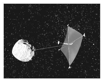
*Figure 5*: Solar sail transport of asteroid. Fleets of solar sails made from lunar aluminum will ply the reaches of the solar system on cargo and research missions. <sup>12</sup>
