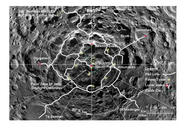
**Figure 1. Circumferential Utilities Network at the Lunar South Pole**. The initial lunar railroad, solar power, communication, and pipeline networks will be placed around the circumference of the Moon at the South Pole. These networks will then be extended to form a global lunar utilities network (Illustration from Schrunk et al.[1]).
