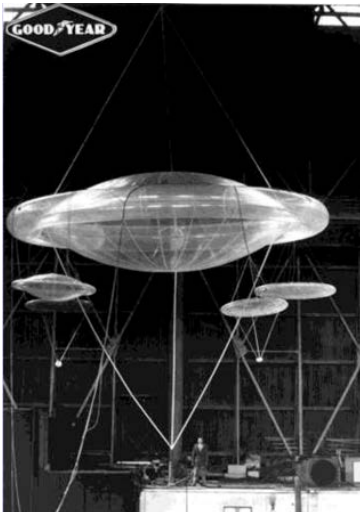
Lenticular Inflatable Parabolic Reflector
