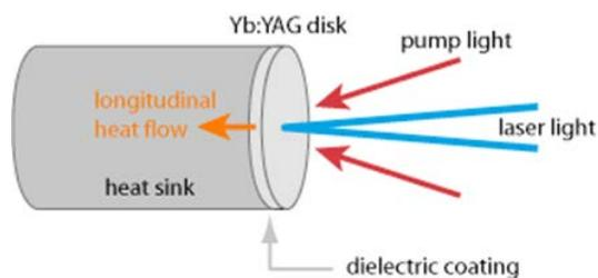
Conjugate optics are set up to recycle reflected pump light 16 times or more in what is known as a multi-pass system. In this way overall efficiency exceeds 80% near the wavelength of the laser's operation.
