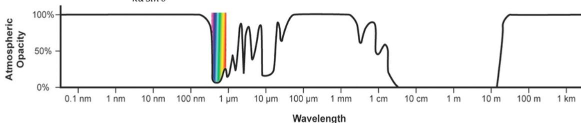
**Short wavelength reduces mass on orbit.** The Earth's atmosphere has sufficient clarity in the microwave, infrared, and visible portions of the spectrum to beam energy reliably from space. At a distance of 35,786 kilometers, the sizes of the transmitting and receiving apertures are fixed by the wavelength used. Using shorter wavelengths reduces aperture diameter and hence the size and mass of the satellite.
