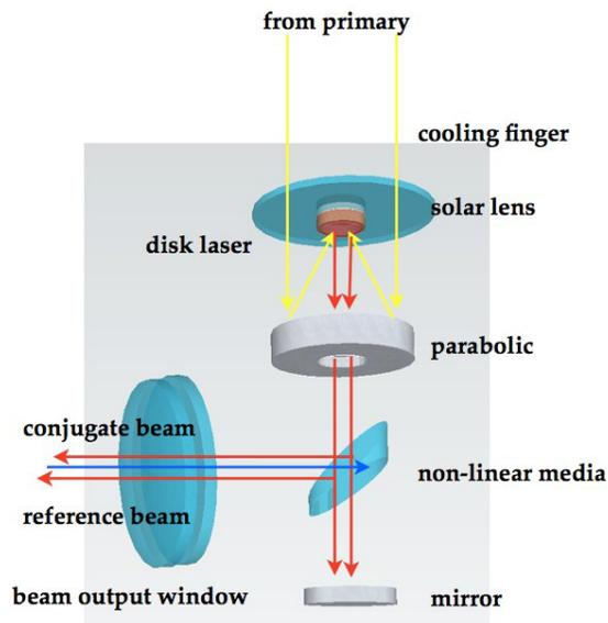
Using these ideas, I have designed a 6,000 meter diameter lenticular parabolic primary concentrator that focuses sunlight 1600x to a solar-pumped thin-disk laser equipped with a 6.6 meter diameter aperture to beam energy to two hundred 6.6 meter diameter receivers on Earth, simultaneously, over a distance of 40,000 km from geosynchronous orbit
