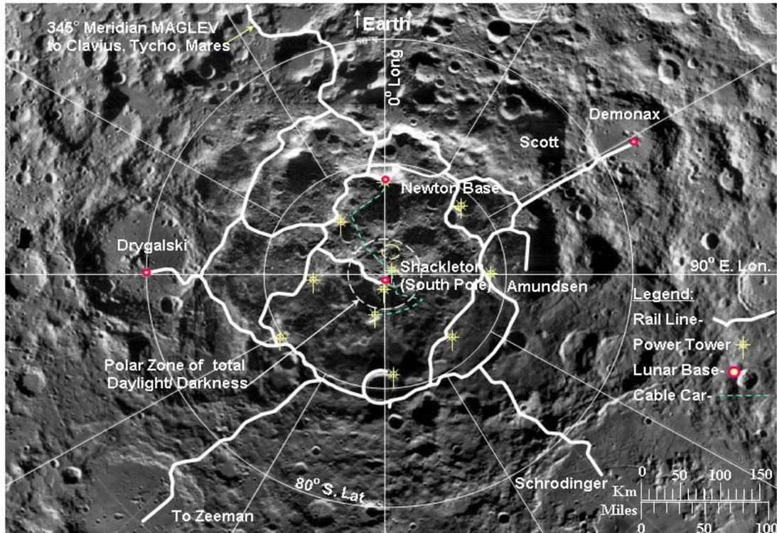
**Figure 1. Circumferential Utilities Network at the Lunar South Pole.** The initial lunar railroad, solar power, communication, and pipeline networks will be placed around the circumference of the Moon at the South Pole. These networks will then be extended to form a global lunar utilities network (Illustration from Schrunck et al.[1]).
